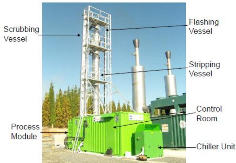
**Figure 9.** Biogas upgrading unit at Motala (unit supplied by Greenlane® Manuka - 80 Nm<sup>3</sup> hour<sup>-1</sup> capacity; Source:www.flotech.com)
