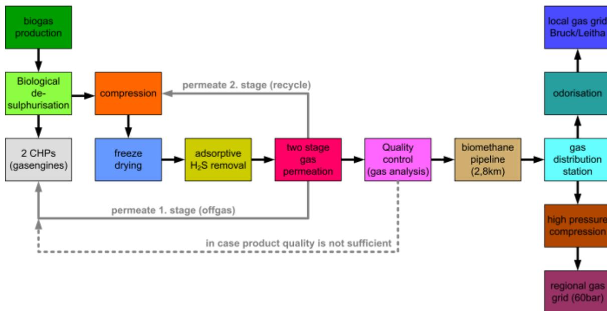
**Figure 6.** Process integration of the biogas upgrading plant Bruck an der Leitha (Source: Virtual Biogas Project, [www.virtuellesbiogas.at](http://www.virtuellesbiogas.at))
