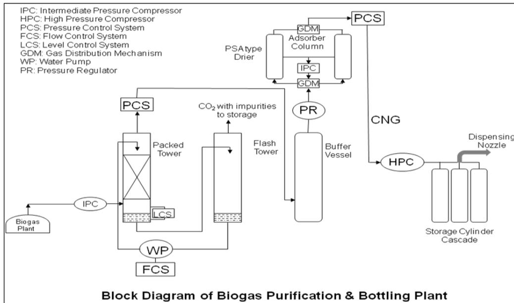
**Figure 11.** Block diagram of the biogas upgradation & bottling plant designed and setup at IIT Delhi campus (source: Prof. V. K. Vijay, IIT Delhi)
