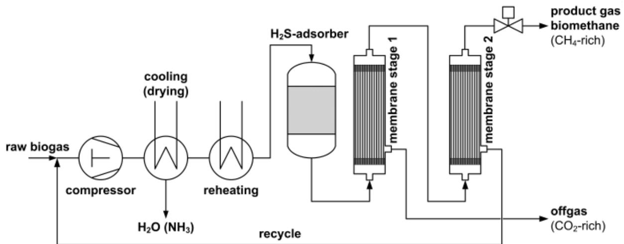
**Figure 5.** Flow sheet of the biogas upgrading plant applying gas permeation in Bruck an der Leitha (Source: Virtual Biogas Project, [www.virtuellesbiogas.at](http://www.virtuellesbiogas.at))
