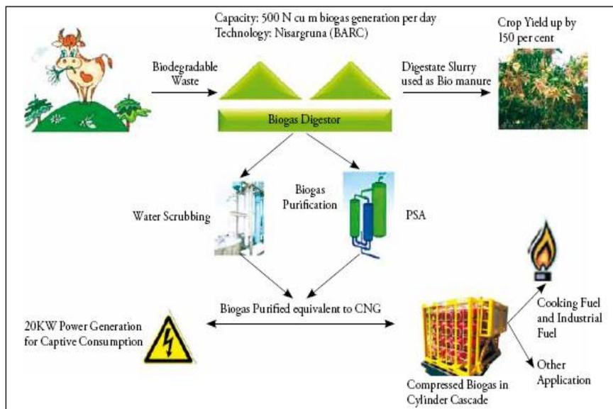
**Figure 15.** Schematic diagram of biogas upgrading and bottling plant at Nasik, Maharashtra (Source: Prof. V. K. Vijay, IIT Delhi, India)
