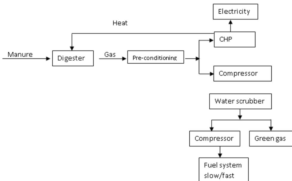
**Figure 2.** Process scheme biogas utilisation at Zalaegerzeg WWTP, Hungary (Courtesy, DMT Environmental Technology, The Netherlands)
