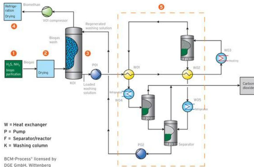
Figure 8. Flowchart of the amine washing process. BCM-Process® licensed by DGE GmbH, Wittenberg (Courtesy: [www.mt-biomethan.com](http://www.mt-biomethan.com))
